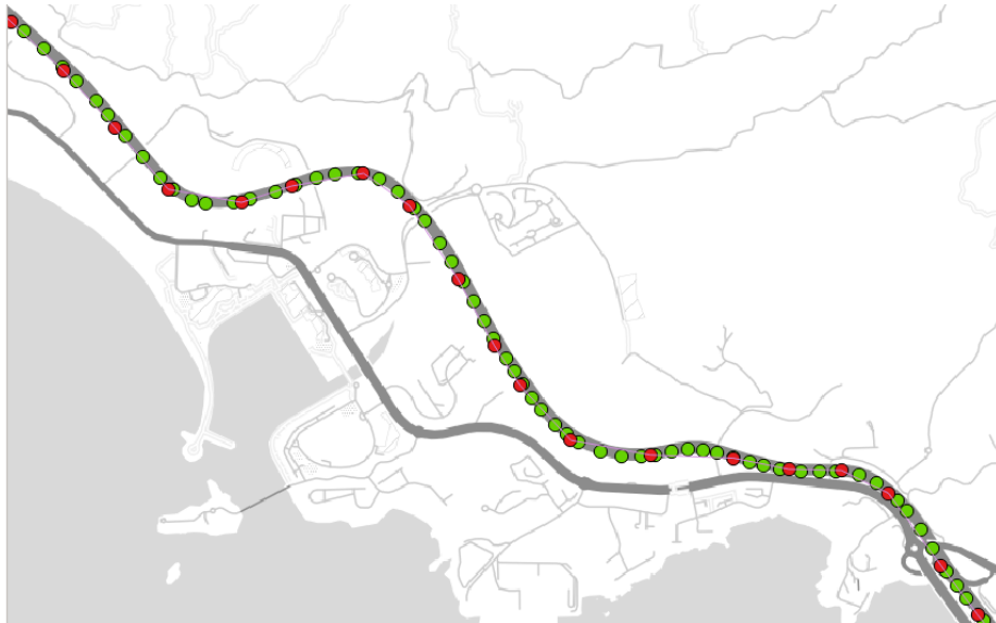
(b) With interpolation this issue can be solved. In this example, red dots stand as GPS observations and green dots in between are observations that are added through interpolation.
